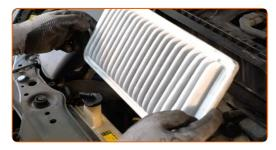
Clean the air filter cover and housing. Use all-purpose cleaning spray.
