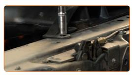
Loosen the fastening clamp connecting the air duct to the air filter housing. Use a drive socket #10. Use a ratchet wrench.
