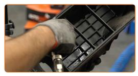
Reinstall the air filter cover. Fasten it.
