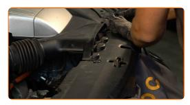
Remove the fender protection cover.
