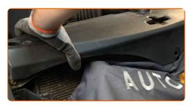
Loosen the air intake fastening. Use a drive socket #10. Use a ratchet wrench.
