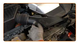
Secure the fastener of the air intake duct. Use a drive socket #10. Use a ratchet wrench.
