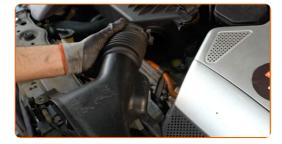
Release the air filter cover clips.
