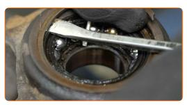
Dismantle the inner bearing race that is remaining on the hub. Use a bush and bearing driver set. Use a bearing separator.
