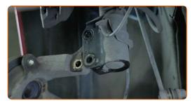
Remove the steering knuckle together with the wheel hub.
