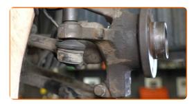
Tighten the fastener that connects the lower arm ball joint to the steering knuckle. Use a combination spanner #16. Use a drive socket #16. Use a torque wrench. Tighten it to 37 Nm torque.
