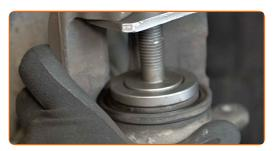
Clean the brake caliper bracket of dirt and dust. Use a wire brush. Use a brake cleaner.
