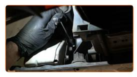
Remove the fuel filter fastening bracket.
