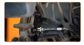
Remove the caliper bracket.
