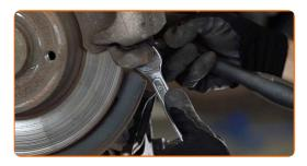
10 Remove the brake caliper.
