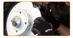
Tighten the brake caliper bracket. Use a drive socket #E16. Use a torque wrench. Tighten it to 105 Nm torque.
