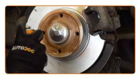
Clean the brake disk surface. Use a wire brush. Use a brake cleaner.
