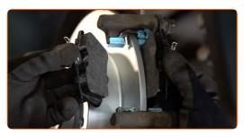
Install the brake caliper and fix it. Use a combination spanner #15. Use a drive socket #13. Use a torque wrench. Tighten it to 35 Nm torque.
