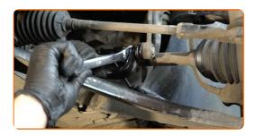
Unscrew the fastener connecting the stabilizer link to the shock strut. Use a drive socket #16. Use a ratchet wrench.
