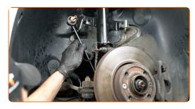
Tighten the fastener connecting the stabilizer link to the stabilizer bar. Use a drive socket #17. Use a torque wrench. Tighten it to 44 Nm torque.
