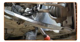
Tighten the fastener connecting the stabilizer link to the shock strut. Use a drive socket #17. Use a torque wrench. Tighten it to 44 Nm torque.
