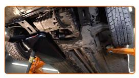
6 Unscrew the drain plug. Use square oil drain plug socket No.8
