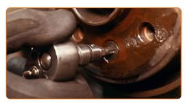
16 Remove the brake disc.
