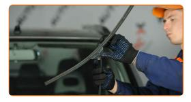
Remove the blade from the wiper arm.
