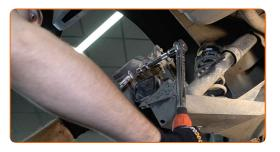
Replacement: wheel bearing – RENAULT TWINGO II (CN0\_). Tip from AUTODOC:
