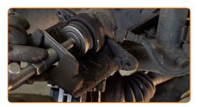
Install the brake caliper and fix it. Use a drive socket #13. Use a torque wrench. Tighten it to 32 Nm torque.
