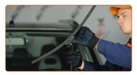
Remove the blade from the wiper arm.
