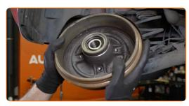
Replacement: wheel bearing – RENAULT Twingo II Box Body / Hatchback (CNO\_). Tip:
