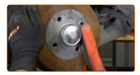
Treat the surface where the wheel rim contacts the brake drum. Use ceramic grease.
