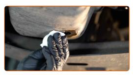
Screw in the new drainage plug and tighten it. Use square oil drain plug socket No.8 Use a torque wrench. Tighten it to 20 nm torque.
