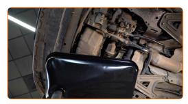
6 Clean the area of the oil pan drainage hole. Use a wire brush.
