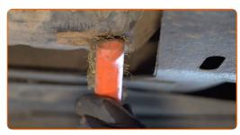
Unscrew the drain plug. Use square oil drain plug socket No.8 Use a ratchet wrench.
