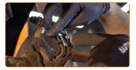
Replacement: brake pads – RENAULT Twingo II Box Body / Hatchback (CNO\_).
