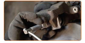
Clean the brake caliper bracket from dirt and dust. Use a wire brush. Use a brake cleaner.
