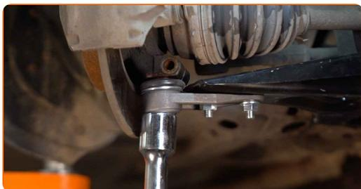
**24** Install the fastening bolt. Use a rubber mallet.
