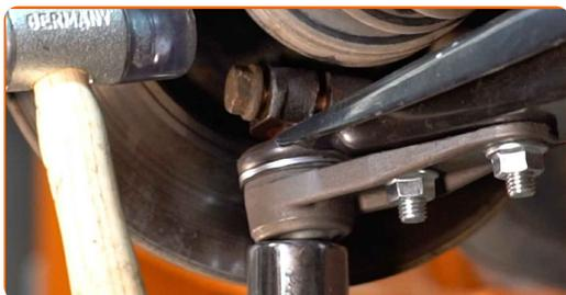
**25** Screw the fasteners of the ball joint. Use a drive socket #16. Use a combination spanner #16.
