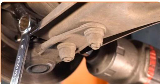
**8** Remove the fastening bolt. Use a rubber mallet.
