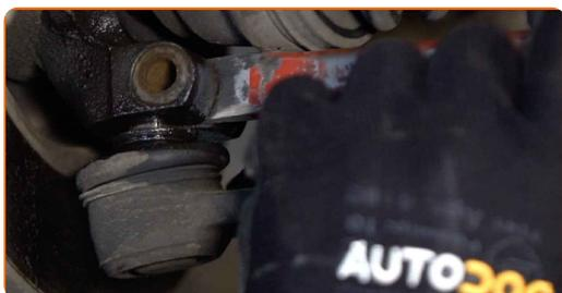
**10** Disconnect the lower arm from the steering knuckle.
