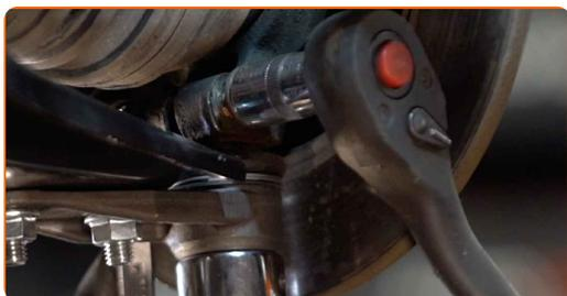
**26** Screw the rear fastener connecting the control arm to the subframe. Use a combination spanner #19. Use a drive socket #19. Use a tap wrench.
