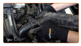
Undo the fastening screws of the air filter cover. Use Torx T25.
