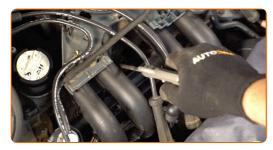
6 Unscrew the spark plugs. Use the spark plug socket #16.
