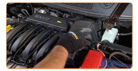
Screw in the air filter box fasteners. Use a drive socket #10.
