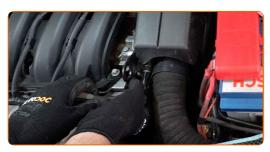
Disconnect the air intake pipe from the air filter box.
