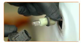
Attach the bulb holder to a new side indicator light.
