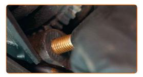
Screw the fastener connecting the ball joint to the steering knuckle. Use a combination spanner #16. Use a drive socket #16. Use a ratchet wrench.
