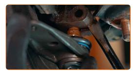
19 Attach the ball joint to the control arm.
