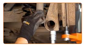
Unscrew the upper fastener of the shock absorber. Use a drive socket #17.
