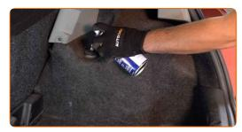
Loosen the upper fastener of the shock absorber. Use a drive socket #17. Use a shock absorber socket DD№6. Use a ratchet wrench.
