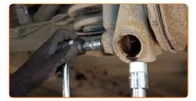
13 Remove the fastening bolt.
