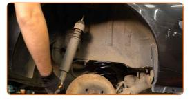
17 Remove the shock absorber mount, boot and bump stop.
