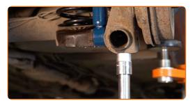
Tighten the lower fastener of the shock absorber. Use a drive socket #18. Use a torque wrench. Tighten it to 105 Nm torque.
