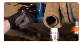
Screw in the lower fastener of the shock absorber. Use a drive socket #18.
