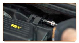
Remove the air filter housing.
