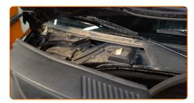
6 Clean the cabin filter housing and cover. Use all-purpose cleaning spray.
