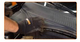
Install the fasteners of the wiper plastic cowl grille. 14
