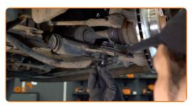
Support the stabilizer bar. Use a hydraulic transmission jack.
