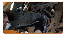
Remove the transmission jack from under the stabilizer bar.
