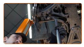
Tighten the stabiliser link fastener. Use Torx T45. Use a drive socket #13. Use a torque wrench. Tighten it to 35 Nm torque.
