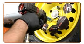
Lower the car and working in a cross order, tighten the wheel bolts. Use wheel impact socket #17. Use a torque wrench. Tighten it to 105 Nm torque.
