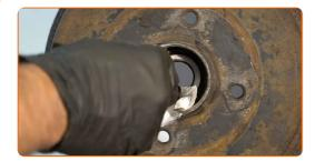
Remove the wheel hub bearing retaining ring. Use circlip pliers.
