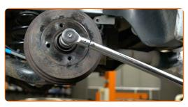
Replacement: wheel bearing – RENAULT Super 5 Hatchback (B40, c40).
