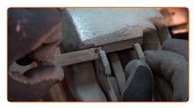
10 Remove the brake pads.
