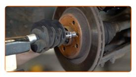
Remove the brake disc.
