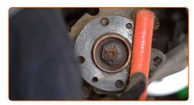
14 Install the new brake disc on the hub and tighten the screws.
