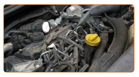
Detach the glow plug wiring connectors.
