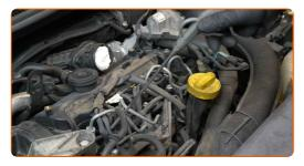
Detach the glow plug wiring connectors.
