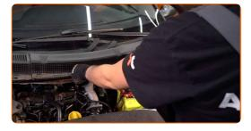
Screw in the fastener of the wiper cowl grille located on the left side. Use a drive socket #10. Use a ratchet wrench.
