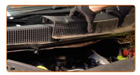
6 Unscrew fixing bolts of the protective cover. Use a drive socket #10. Use a ratchet wrench.
