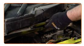
Tighten fixing bolts of the protective cover. Use a drive socket #10. Use a ratchet wrench.
