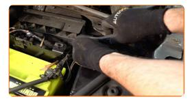
Raise a little the top protective cover. Remove the air filter housing.
