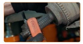
Clean the ball joint mounting seat. Use a wire brush. Use WD-40 spray.
