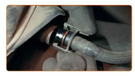
Clean the fasteners on the air filter housing. Use all-purpose cleaning spray.
