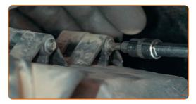
9 Remove the air filter housing.
