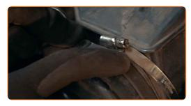
Screw the fastening clamp connecting the air duct to the air filter housing. Use a drive socket #7. Use a tap wrench.
