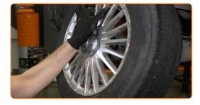
Remove the hub bearing cap. Use a crowbar. Use a hammer.
