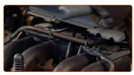
Remove the spark plug wire connectors from the spark plug wells. Use round-nose pliers.
