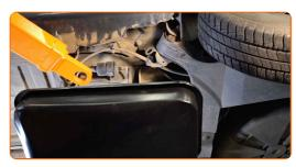
Squeeze the clips and detach the fuel supply lines from the fuel filter housing. Use fuel line pliers.
