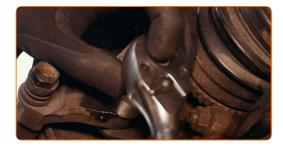
Remove the caliper bracket.
