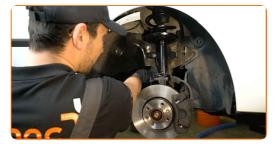
Treat the shock strut fasteners. Treat the fasteners of the ball joint. Treat the fastener connecting the tie rod end to the steering knuckle. Use copper grease.
