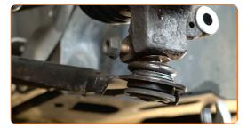
Screw the fasteners of the ball joint. Use a combination spanner #16. Use a drive socket #16. Use a tap wrench.
