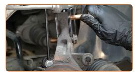
Disconnect the steering knuckle from the shock absorber strut.
