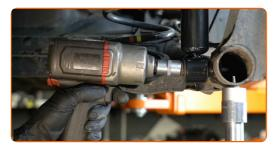
10 Remove the fastening bolt.
