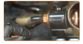
Connect the ABS sensor wiring.
