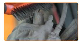
Unscrew the brake caliper fasteners. Use a combination spanner #13. Use a combination spanner #15.
