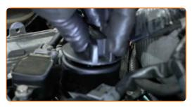
77 Tighten the oil filler cap.
