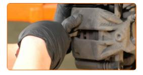
Remove the brake caliper.
