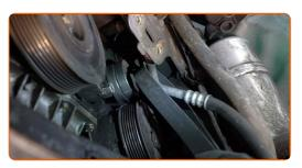
Replacement: serpentine belt – RENAULT Megane III Hatchback (BZ0/1\_). Tip from AUTODOC:
