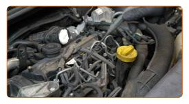
Detach the glow plug wiring connectors.
