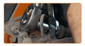
g Remove the brake caliper.
