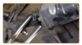
Replacement: fuel filter – RENAULT Megane III Box Body / Hatchback (BZ\_).
