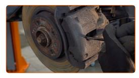
10 Remove the brake caliper.
