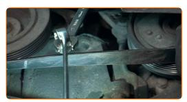
Place the V-ribbed belt on the tensioner pulley. Return the tensioner pulley to its initial position.
