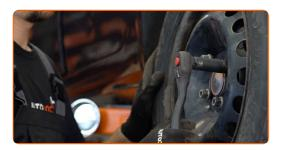
Lower the car and working in a cross order, tighten the wheel bolts. Use a torque wrench. Tighten it to 110 Nm torque.
