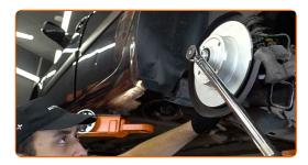
Treat the hub where it contacts the brake disk. Use a multipurpose grease.
