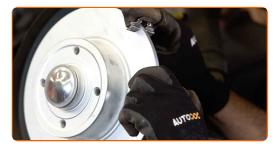
Tighten the brake caliper bracket. Use a drive socket #E16. Use a torque wrench. Tighten it to 105 Nm torque.
