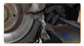
10 Remove the brake caliper.
