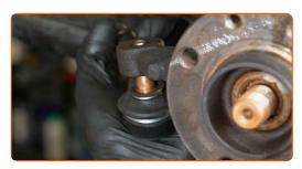
Screw on the fastening nut that connects the tie rod end to the steering knuckle. Use a drive socket #17. Use a ratchet wrench.
